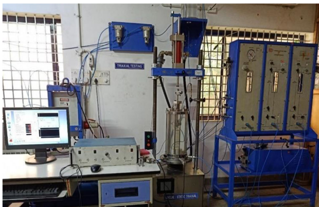
Fig. 8 Cyclic triaxial apparatus used for the present study (Courtesy: Sarathy Geotech Lab Pvt.Ltd)
