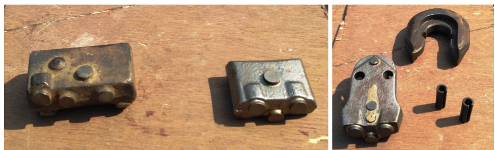
Fig. 9 Replaceable teeth blocks
