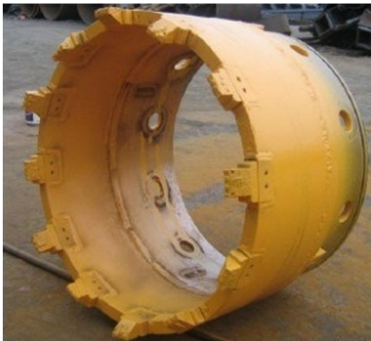
Fig. 8 Double-walled casing—casing shoe with replaceable teeth blocks
