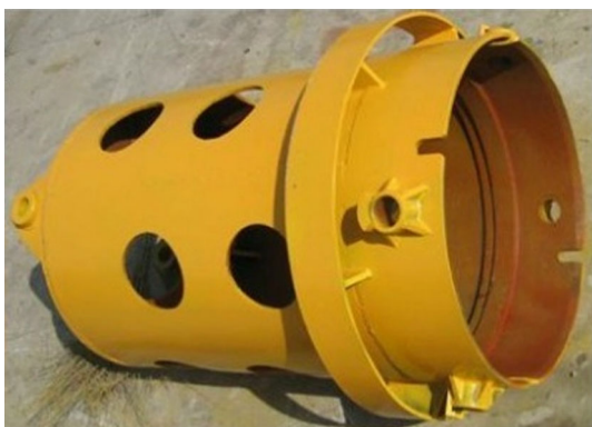
Fig. 6 Double-walled casing—casing adapter
