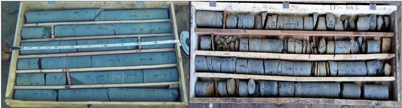
Fig. 4 Cores recovered during preconstruction borehole investigations (BH-01—left and BH-02 right)
