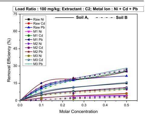
state, due to which  $PbCO_3$  and  $PbSO_4$  get precipitated when level of heavy metal contamination crosses the level of solubility of hydroxides and carbonates at a given pH [87, 88]. Hence, it can be understood from the desorption tests of individual heavy metals that enzyme treatment is effective in reducing hazardous effects of heavy metal contaminants.
