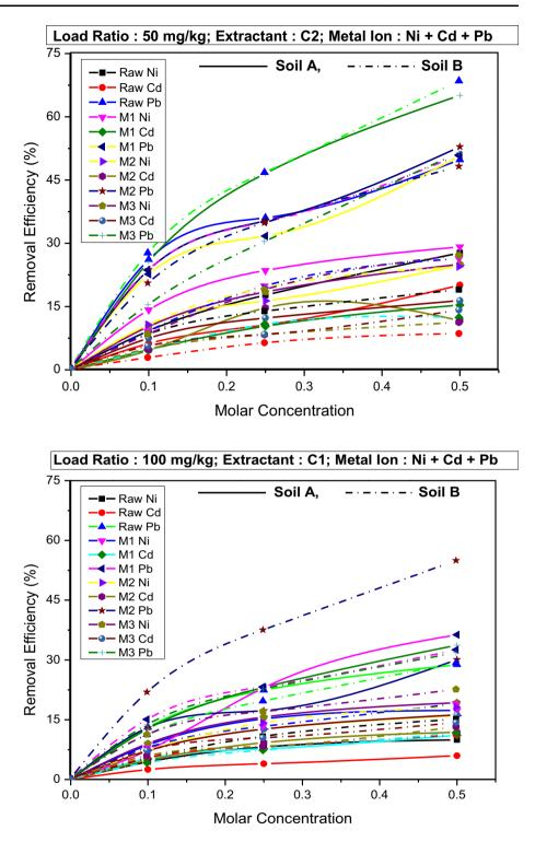
**Fig. 6** Removal efficiencies of Ni, Cd, and Pb spiked together in both soils extracted using C1-EDTA (100 mg/l)
