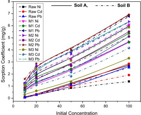
at a pH of 5.85 for 1:100 dilution ratio, sorption coefficient of untreated Soil B was 5.50383 mg/l for 1:100 dilution ratio at pH of 6.11. It is evident that soil treatment with enzyme solutions boosts the capacity of soil grain surfaces to create sites for heavy metal ions to occupy.
