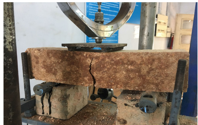
Fig. 5 Failed sample during the flexure test
