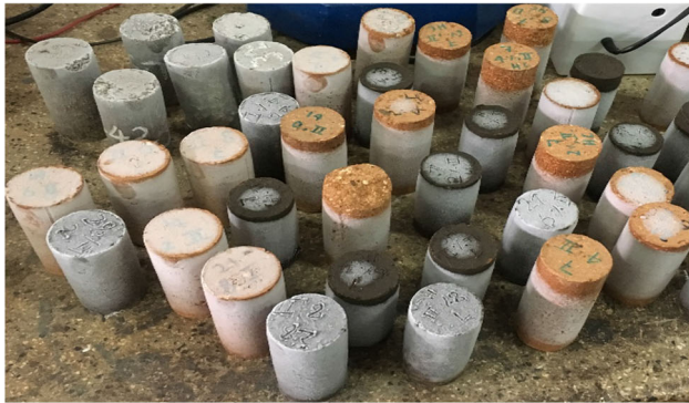
(b) Samples were taken out from freezer during FT test.
