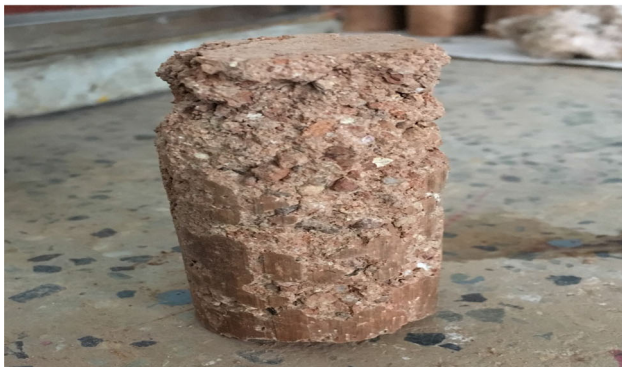
(c) Durability sustained sample after 12 cycles of the WD test.
