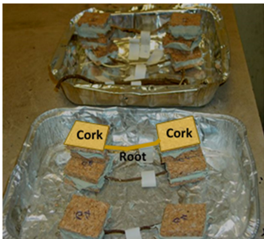
Fig. 9 Root samples utilized for tensile tests and equipped with cork clamps
