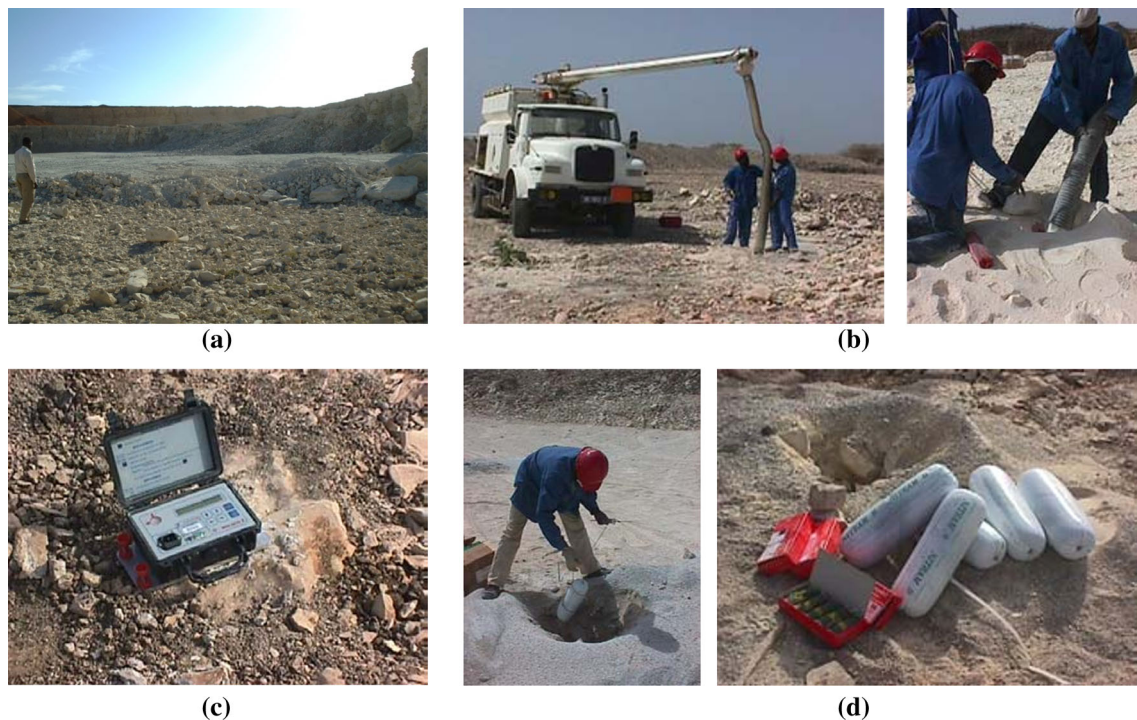
Fig. 3 a “Sococim cement factory.” b, d Drilling of TNT filling inside the boreholes. c “Mini seis” device
