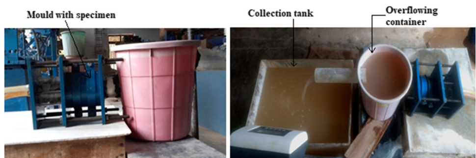
Fig. 1 Schematic diagram of the hole erosion test setup
