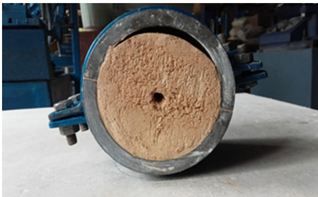
Fig. 16 Sample which collapsed when compacted to 90% wet of optimum
