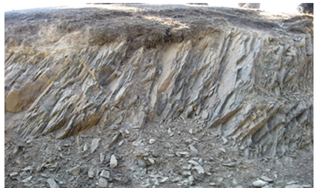
Fig. 40 Thinly foliated meta siltstones of Hasthoji Formation showing high weathering close to surface
