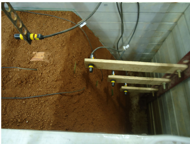
Fig. 4 Photograph of model slope of 75° with instrumentation
