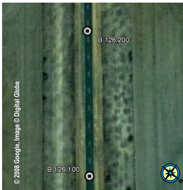
Fig. 7 Aerial image of Borung Highway, 126,100–126,200 m that contains evidence of Gilgai relief in the road reserve (Google Earth dated 16th April, 2008)
