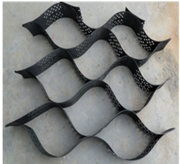
Fig. 3 Typical geocell mattress used in the study
