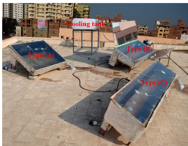
Fig. 2 Photograph for the different designs of tested single-slope solar stills
