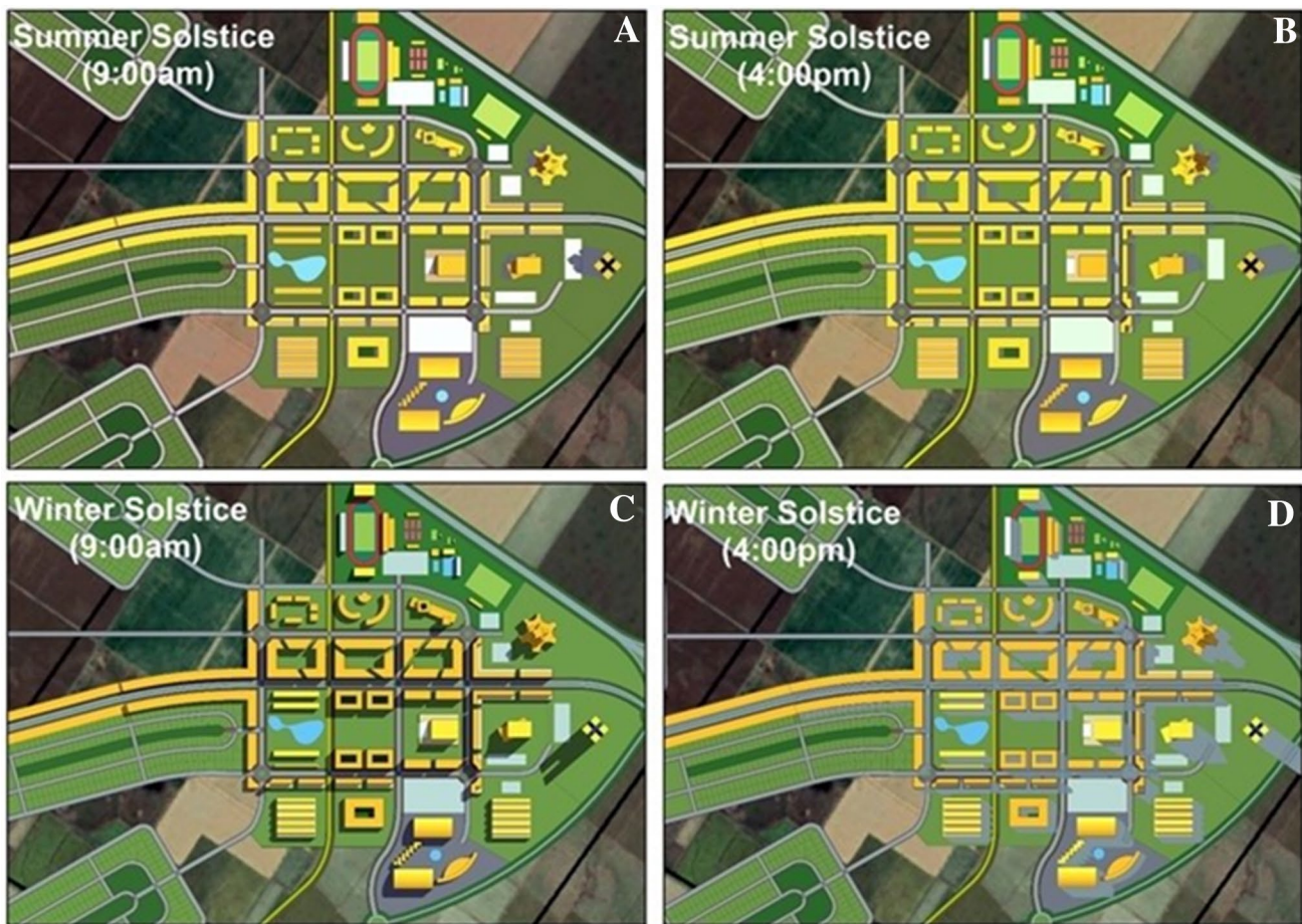
Fig. 12 Shadows produced during working hours (9 a.m. and 4 p.m.) for summer and winter solstices
