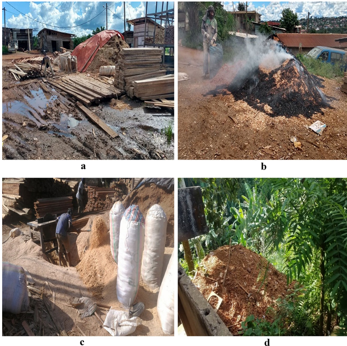
Fig. 8 Popular methods of sawdust disposal (a) Heaps blocking runoff (b) Burning (c) Digging out machine overwhelmed by sawdust (d) In bushes
