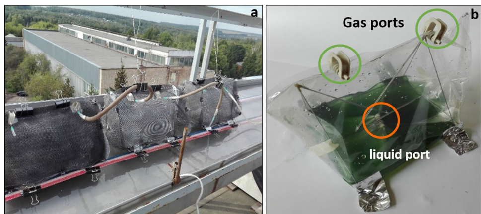
Fig. 2 Experiment #2: two out of three initial PhBRs were in operation (a), single bag with culture (b)
