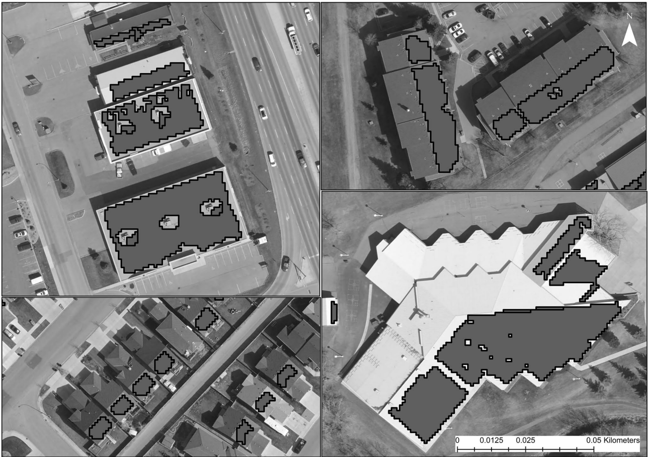
Fig. 5 Examples of suitable rooftop area selection (roof applications such as chimneys have been excluded)
