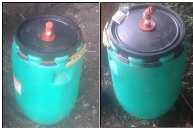
Fig. 2 Air tightness test for TSF
