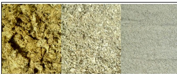
Fig. 1 Size of pineapple waste textures, from left: coarse, medium, and fine
