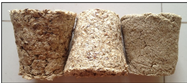
Fig. 4 Surface texture of decomposable pots, from left: coarse, medium and fine
