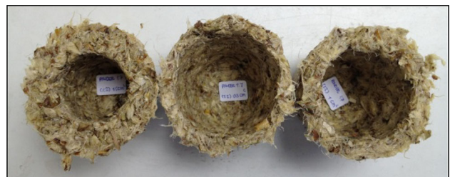
Fig. 2 Thickness of decomposable pots, from left: 1.5, 0.5 and 1.0 cm
