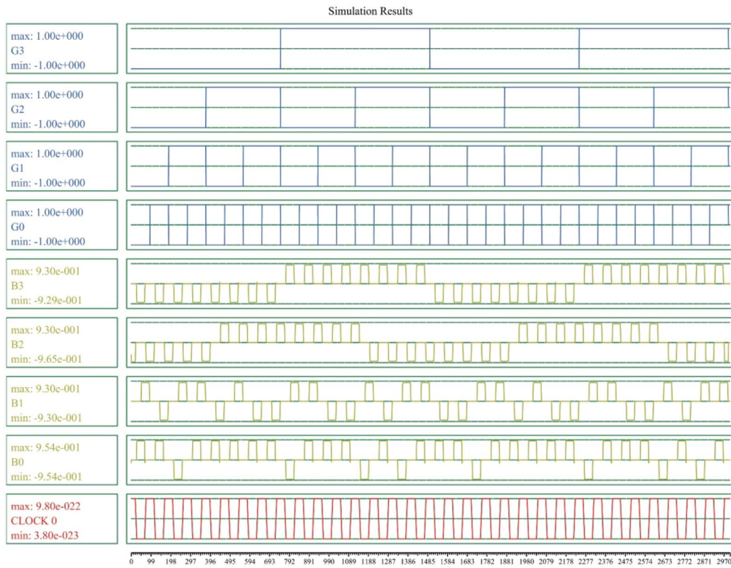
Fig. 14 Obtained outputs from the proposed circuit to convert Gray code to binary
