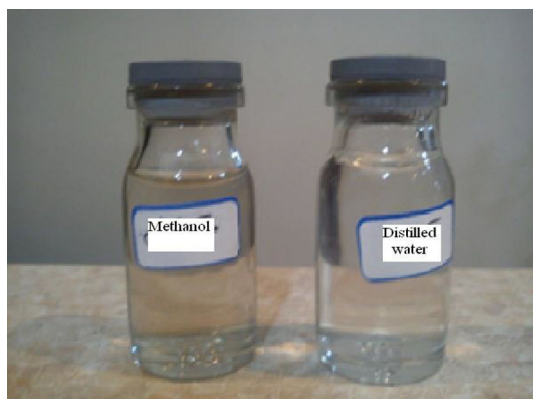
Fig. 1 Zn and ZnO nanoparticles solution generated by 1064 nm laser pulse wavelength in methanol and water after production
