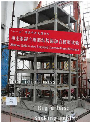
Fig. 10 RAC frame tested.
