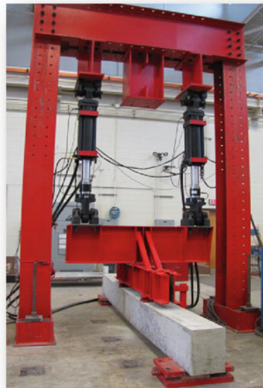
(c) Test setup and load pattern Fig. 2 Load pattern and location of strain gauges on the test beams.
