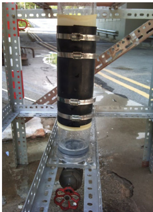
Fig. 2 Water permeability test set-up.
