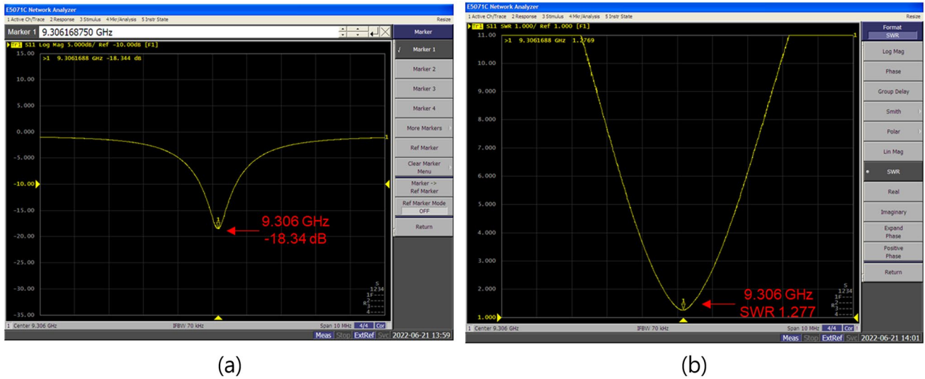
Fig. 10 Measurement of X-band LINAC characteristics with network analyzer: (a) S11, (b) SWR
