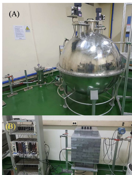
Fig. 4 A Manganese-sulfate bath system with 1000 L of ^{55}\text{MnSO}_4 solution (A) and two NaI(Tl) detectors within a lead shielding box with a data acquisition system (B)
