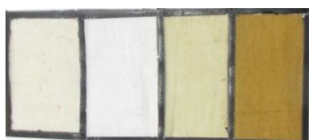
Fig. 2 Colour development on Cotton Khadi by application of Anar peel
