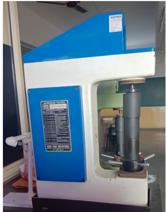
Fig. 4 Brinell Hardness tester setup for Hardness Evaluation
