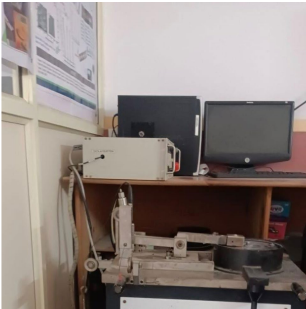
Fig. 3 Tribological wear testing machine (Pin-on-disk setup)
