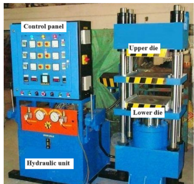
Fig. 1 Hydraulic-assisted compression molding setup
