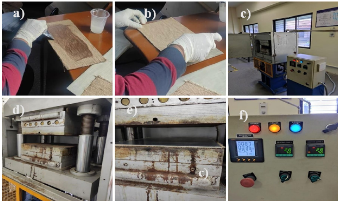
Fig. 3 a, b Hand-layup process of FFAL. c The compression moulding apparatus. d The compression and heater plates inside the apparatus. e The material is kept inside the apparatus and a pressure of 30 bar is applied. f The heaters are heated to 70 °C and then left for 4 h
