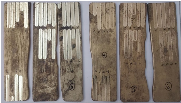
Fig. 7 Cu-Al-Mn SMA alloy samples after milling operation
