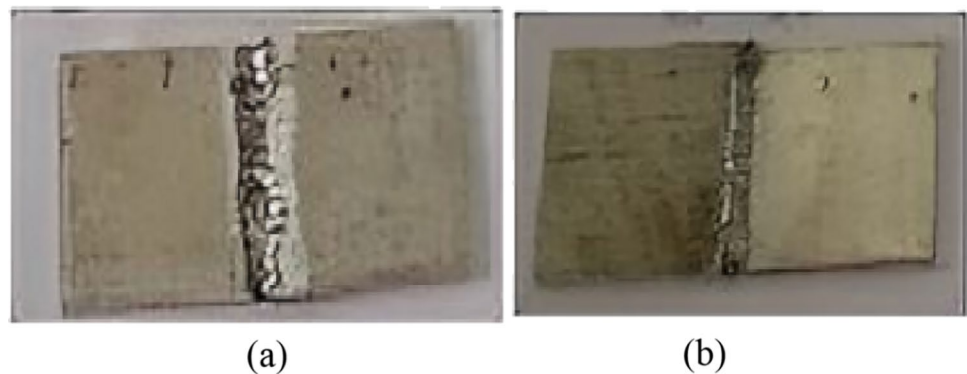
Fig. 3 Samples after welding a without flux and b with \text{TiO}_2 flux
