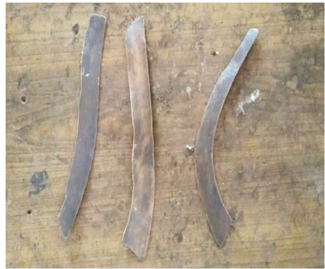
Fig. 3 Hot-rolled samples of CAM1, CAM2 and CAM3 ternary SMAs
