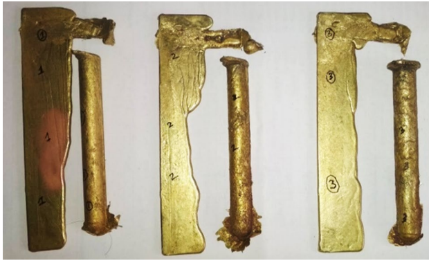
Fig. 2 As-cast samples of Cu–Al–Mn ternary SMAs
