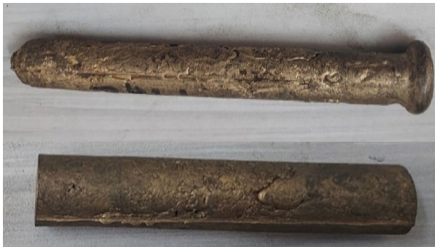
Fig. 6 Cylindrical specimen of CAM3 ternary SMA
