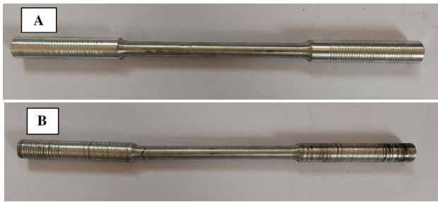
Fig. 2 Fatigue test specimens, A—Before testing, B—After testing
