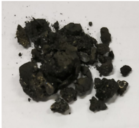
Fig. 4 EAFD – coal composite pellet, containing C/O molar ratio of 1, reduced at 1200°C under flash heating
