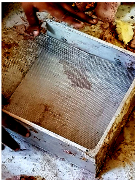
Fig. 2 Die setup coated with wax for fabricating organic PU foam
