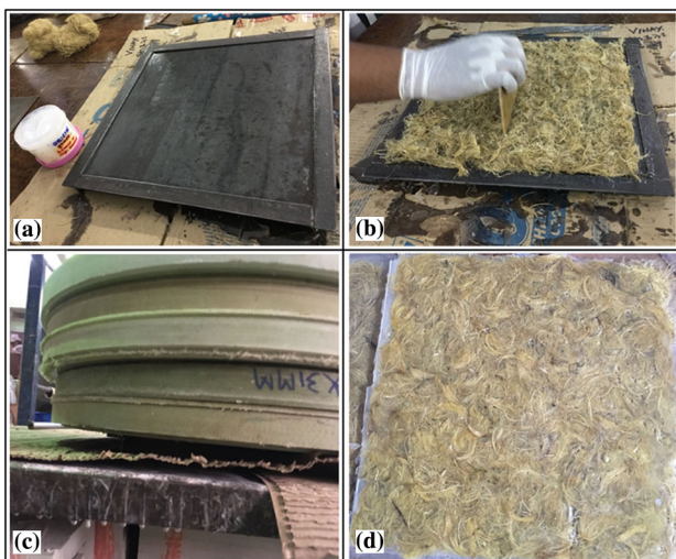
Fig. 3 a Waxing of mould, b random arrangement of fibre in mould, c application of uniformly distributed load on mould and d unmoulded composite panel
