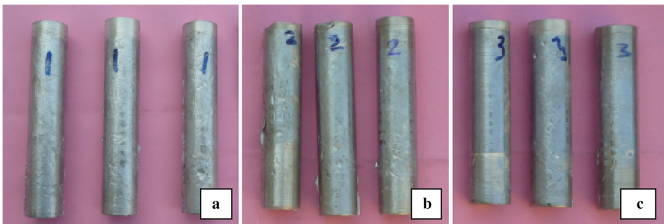
Fig. 4 Samples prepared from composite with 7 wt% of Al 2 O 3 : a 10% SiC, b 15% SiC, c 20% SiC
