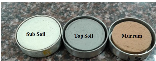
Fig. 5 Shrinkage property of mine overburden material
