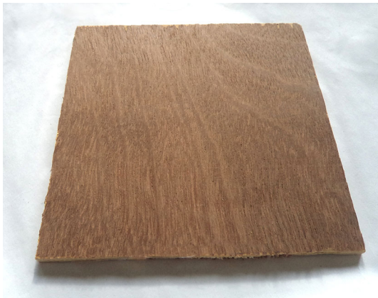
Fig. 2 Shows a plywood sample after test and it is not damaged
