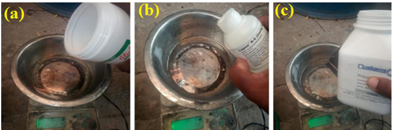
Fig. 4 Chemicals used in the study a epoxy resin—LAPOX L-12, b hardner—Lapox K6, c releasing agent—polyvinyl alcohol]
