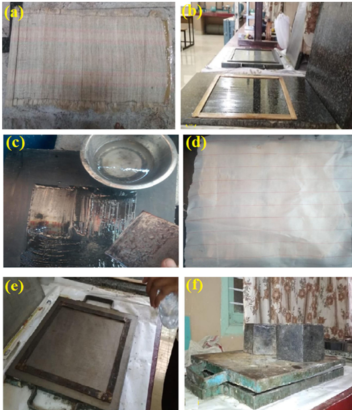
Fig. 5 Stepwise procedure followed in the study for preparation of composites by hand layup process a fibre mat, b releasing agent applied on the surface, c resin application, d application of insulating paper, e alternative layers of fibre and resin placed, f load applied
