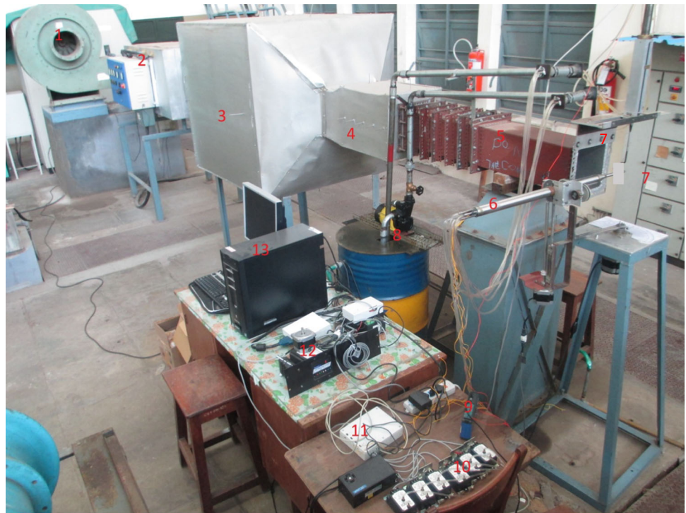
Fig. 9 Photograph of high-temperature calibration facility (HTCF)
