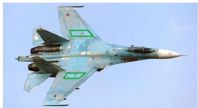
Fig. 11 The most critical zones on airplane structure
