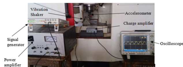
Fig. 15 Experimental set up for modal testing of the spindle tool unit
