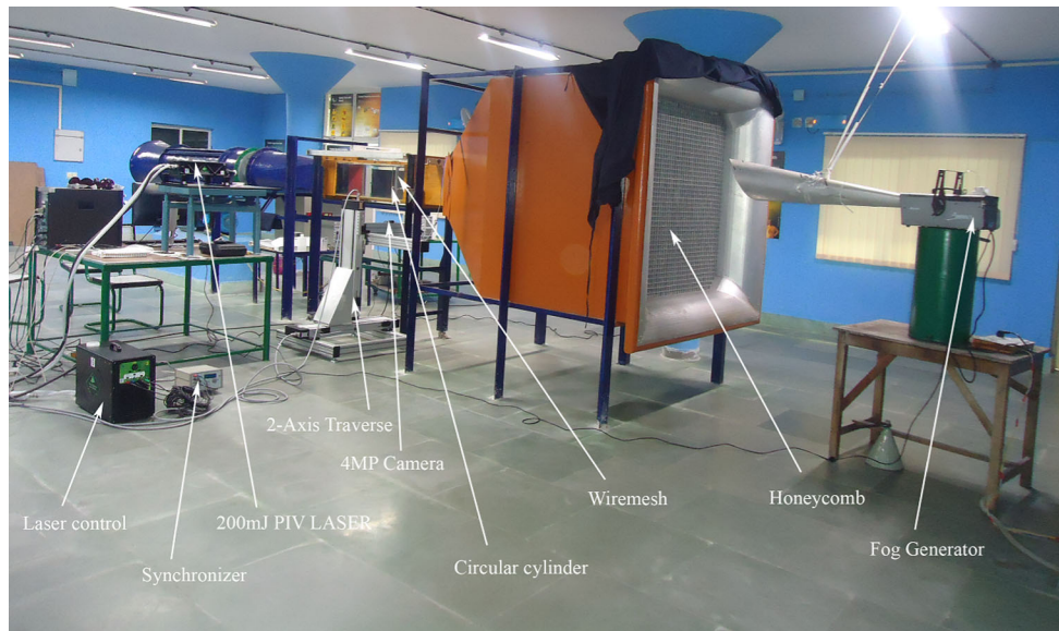
Fig. 1 Open circuit wind tunnel with experimental setup and apparatus
