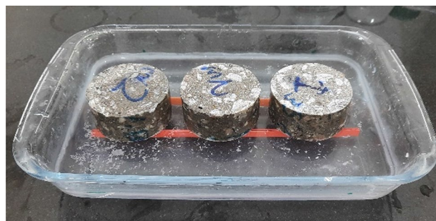
Fig. 2 Samples for water sorptivity testing stored in saturated calcium hydroxide solution
