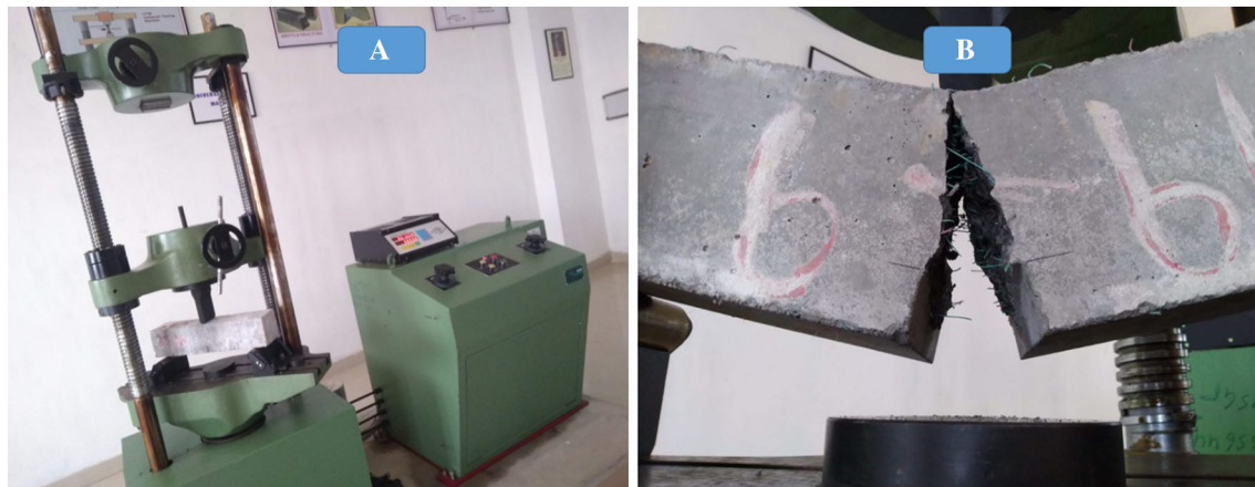
Fig. 9 CMOD flexure test: a Three-point load set up; b Fiber bridging action and failure pattern
