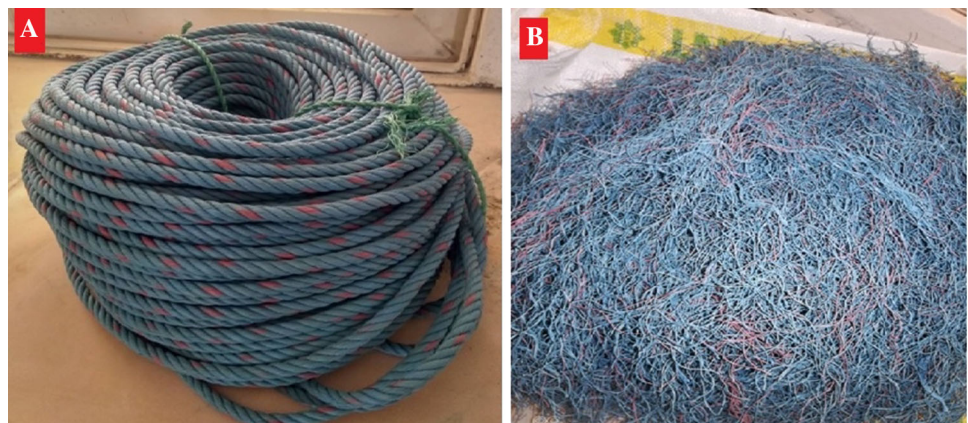
Fig. 2 Photographs of rHDPE: a rope before cutting, b after cutting as the fiber
