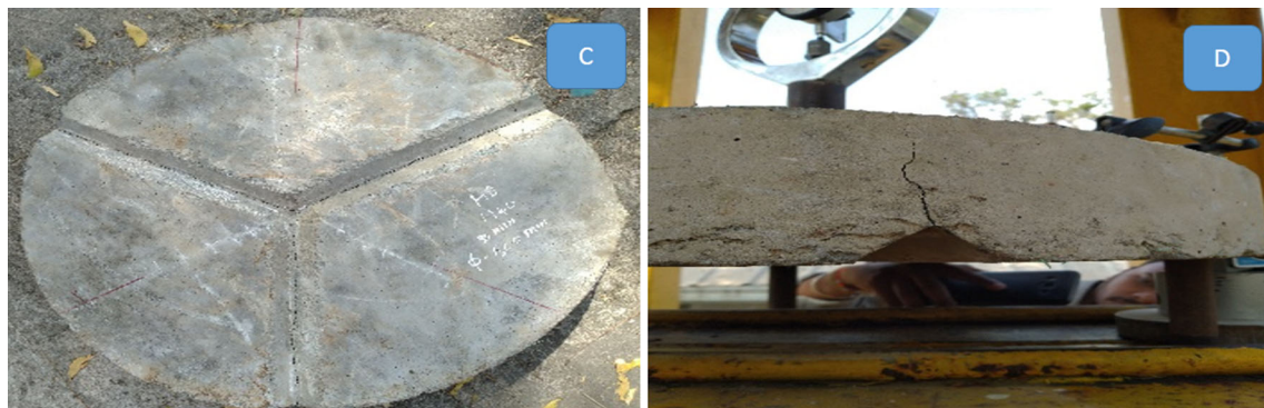
Fig. 12 Failure pattern of round determinate slab test (RDST)
