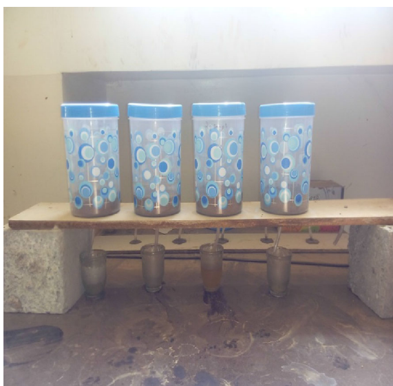
Fig.2 Arrangement of leaching test for solidified soil
