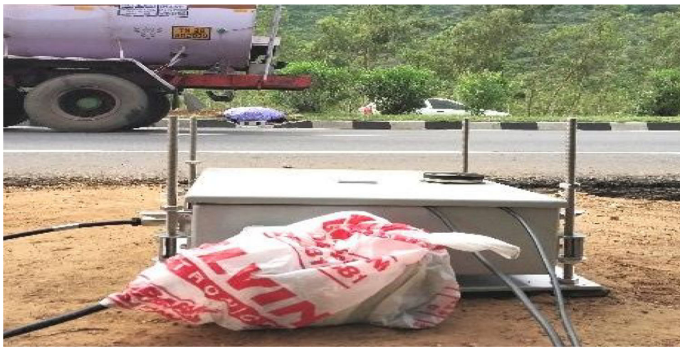
Fig. 2 Set up of IR sensor detector device across NH-32
