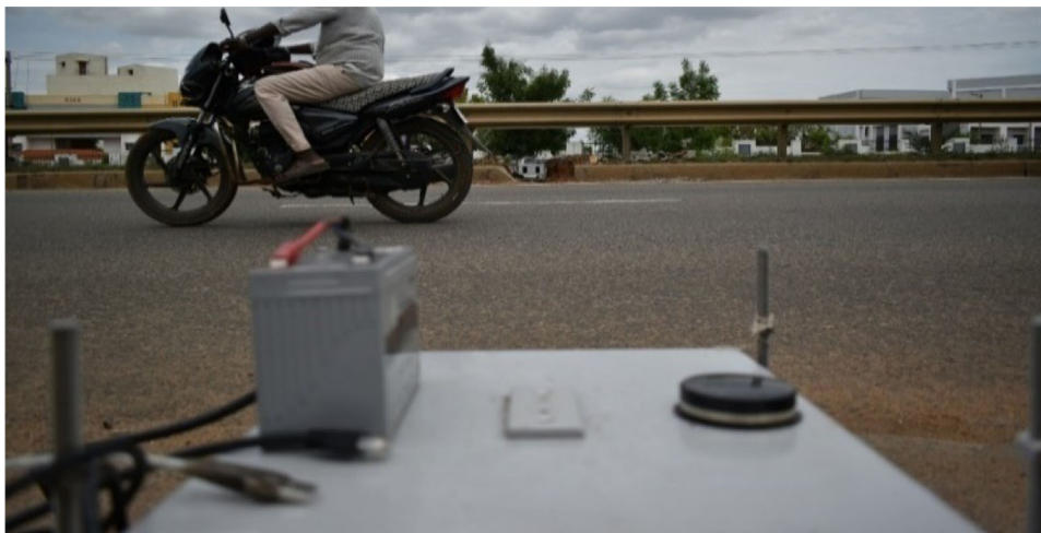
Fig. 4 Set up of IR sensor detector device across NH-83
