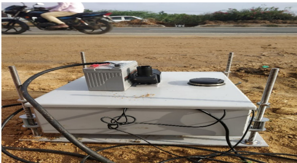
Fig. 3 Set up of IR sensor detector device across NH-38
