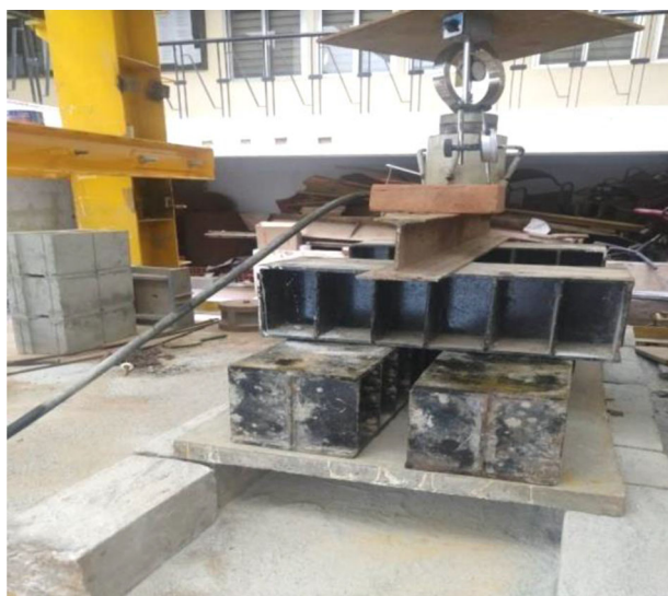
Fig. 3 Test set-up of one way slab
